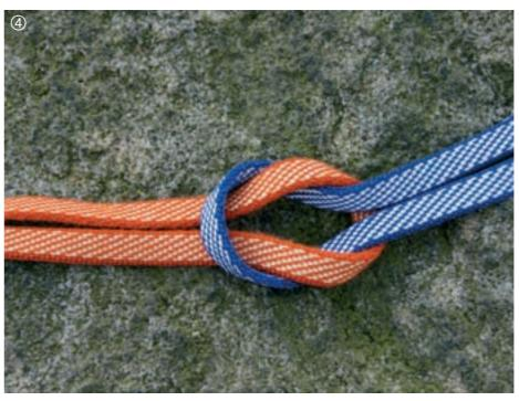
50%. Again this weakening is much more pronounced in Dyneema and especially in the new breed of super skinny 8mm Dyneema slings.
